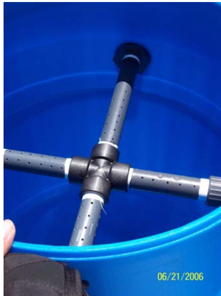
Figure 7 Filter Drum Manifold
