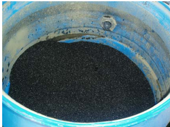
Fresh Activated Carbon (8/24/06)
